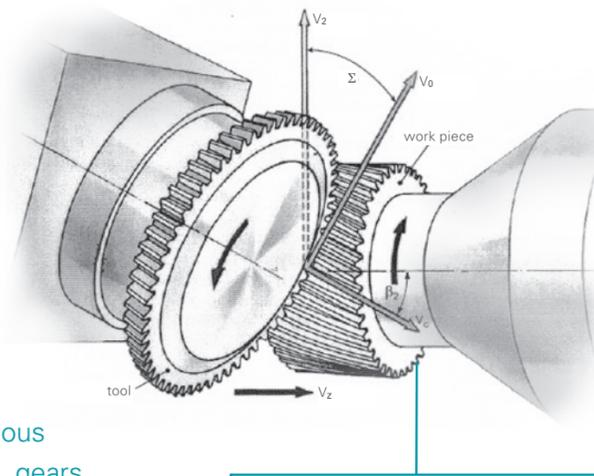
In power skiving, the workpiece and tool form a type of cross-helical gear box.
