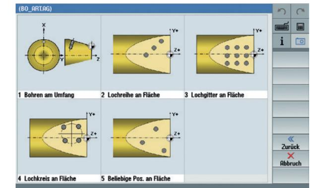
Progressively detailed dialog boxes for machining selection "drilling on an inclined surface".
