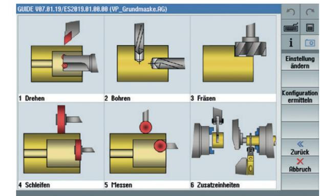
Identical screens on all machines for starting the programming of a machining sequence.
