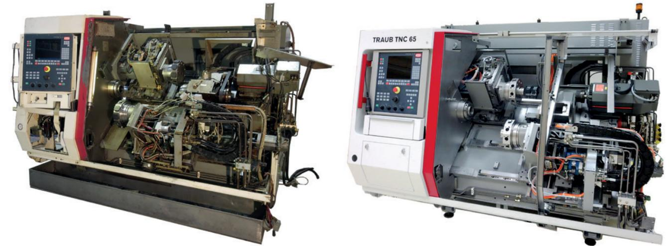
How the nearly twelve-year-old TNC65 looked before the refit. After the refit, the machine not only looks as good as new – it is also at least as accurate as it was on initial delivery.
